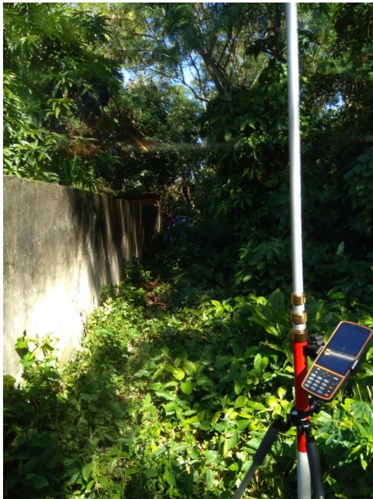
Figura 04: GNSS “rover” (receptor móvel)
